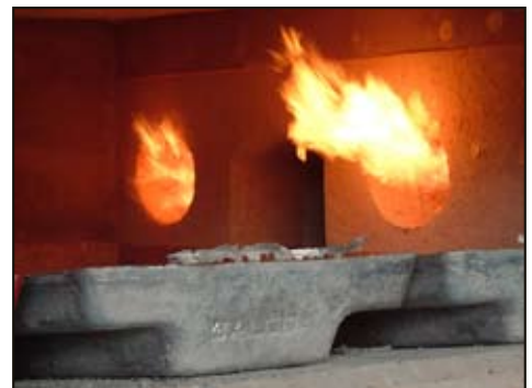
Furnace lining after one week of work start-up for ingot casting
