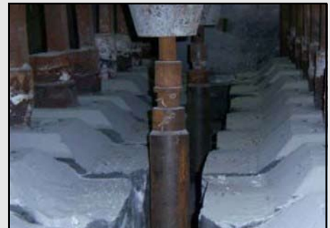
Crust breakers are used in "Prebake Anode Reduction Cells" whereas Soderberg pots are not equipped with point feeders for making alumina additions.
